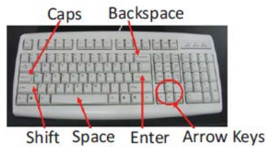
Fig.6.2.2. Parts of a Keyboard
